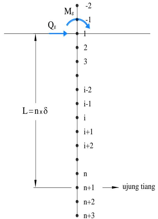
Figure 1 Finite Difference Method for Laterally Loaded Pile
