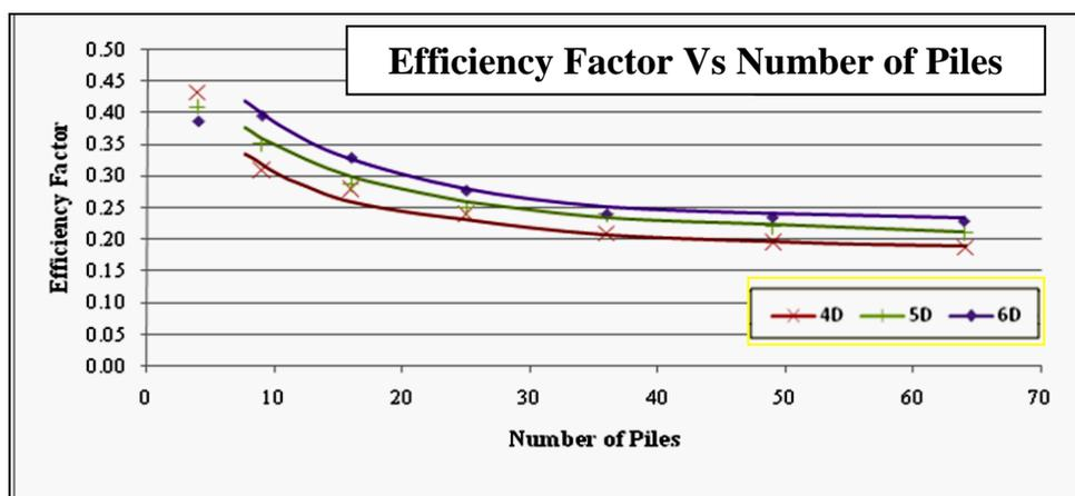
Figure 6 Efficiency Factor vs Number of Piles based on Plaxis Analysis
