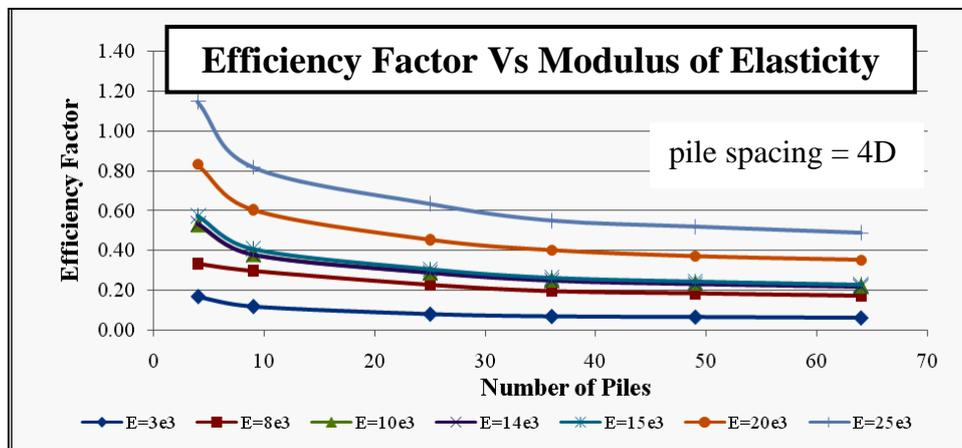
Figure 7 Influence of Soil Stiffness Modulus for Symmetrical Pile Configuration; E = Soil Stiffness Modulus in  $\text{kN/m}^2$
