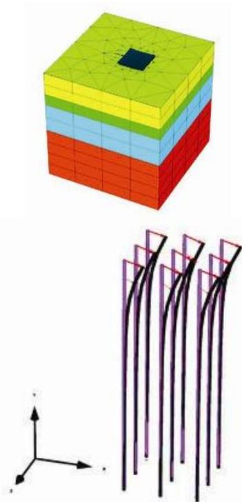
Figure 4 Output of Plaxis 3D Foundation For The Group of 9 Piles
