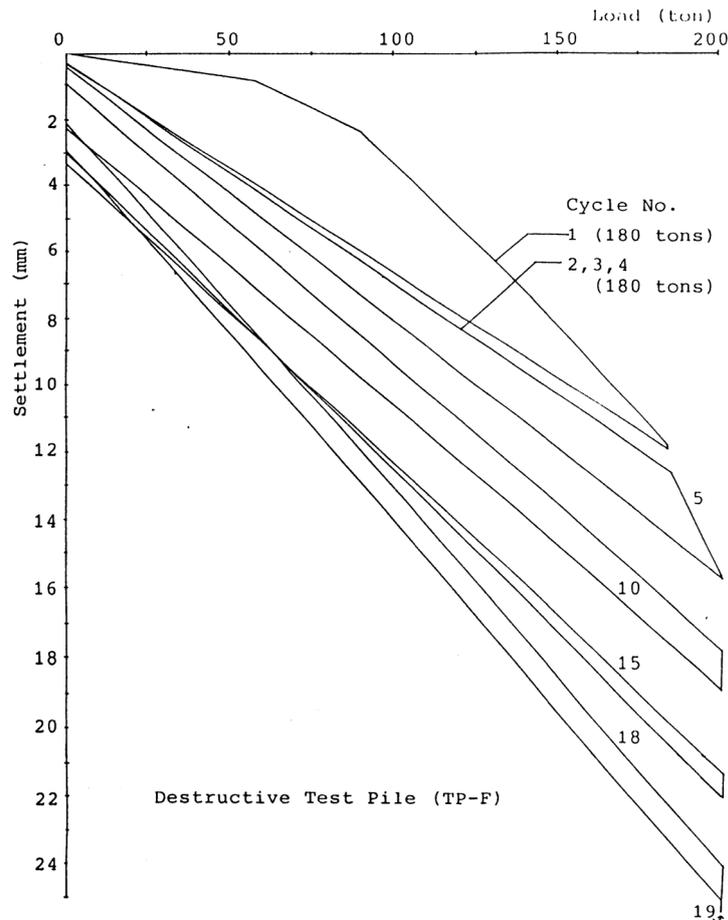
Fig. 6 Load Settlement Curve of Destructive Pile Test (1 ton  $\approx$  10 kN)
