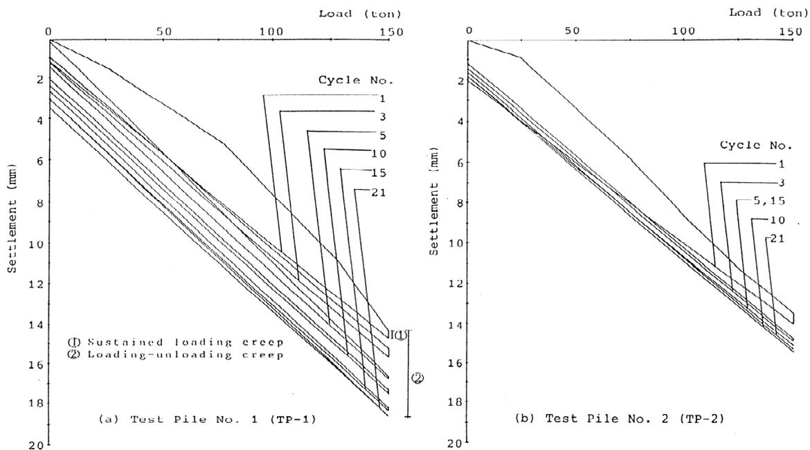
Fig. 5 Load Settlement Curve of the Proof Test Piles (1 ton  $\approx$  10 kN)
