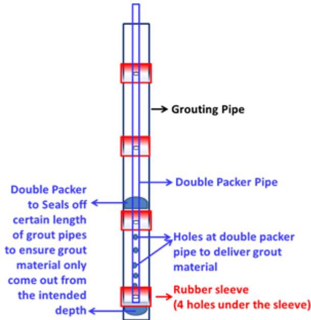
Fig.1 Tube a Manchette (TAM) Grouting System
