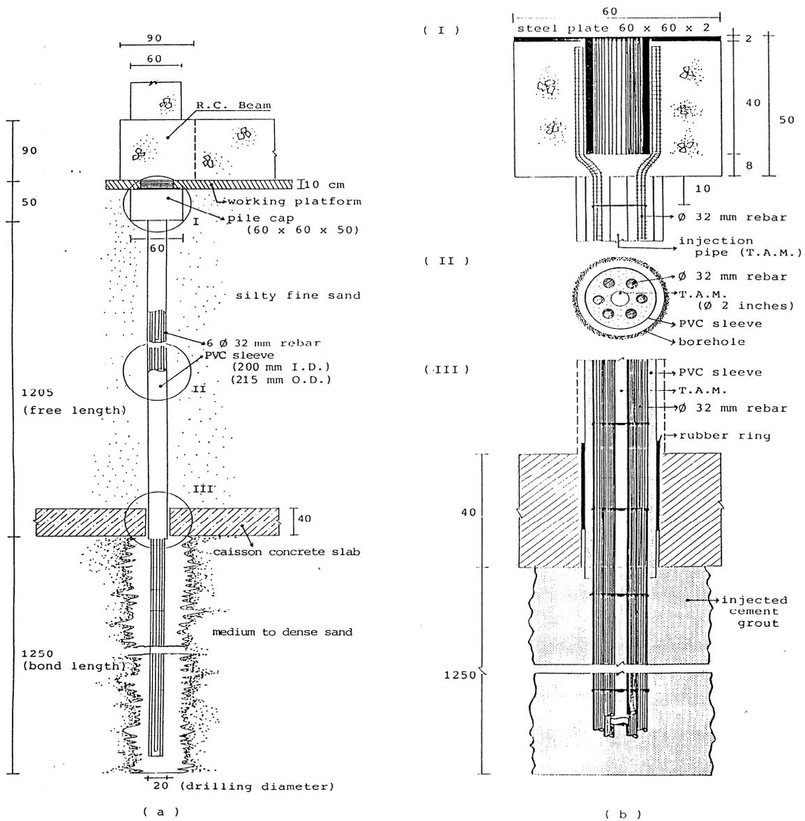
Fig. 3 Detail Construction of the Repetitive Grouted Micropiles (RGM)
