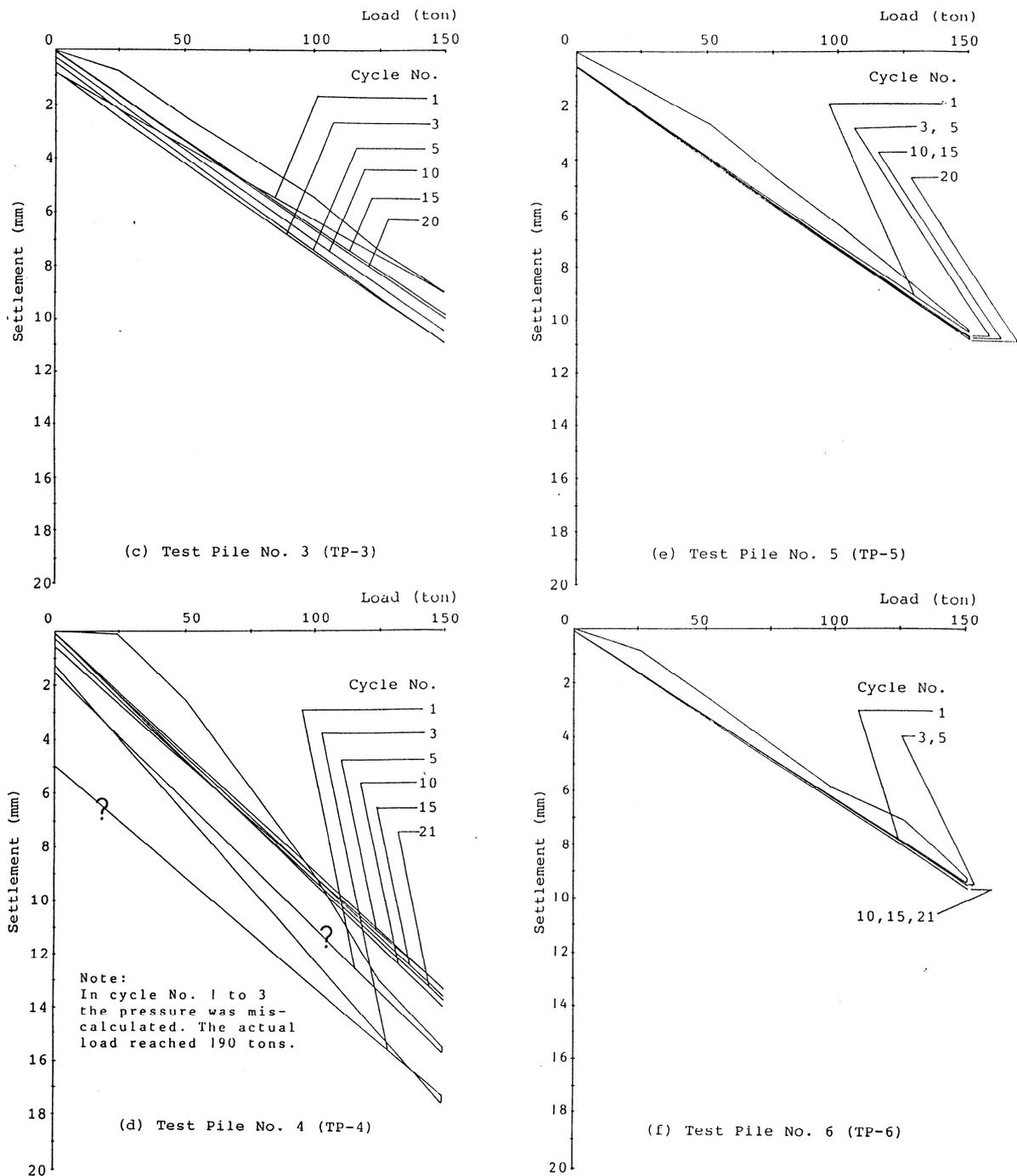
Fig. 5 (con't) Load Settlement Curve of the Proof Test Piles (1 ton  $\approx$  10 kN)
