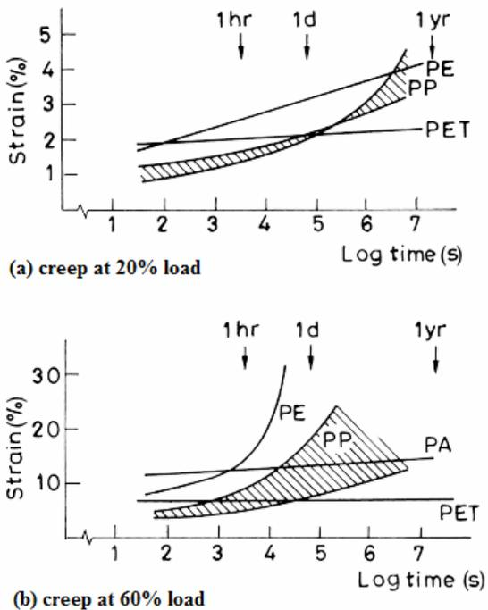
Figure 10. Results of Creep Tests on Various Yarns of Different Polymers (after den Hoedt, 1986; from Shukla and Yin, 2006)
