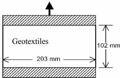
(b) Wide-width Tension Test (ASTM D 4595)
