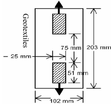
(a) Grab Tensile Test (ASTM D4632)
