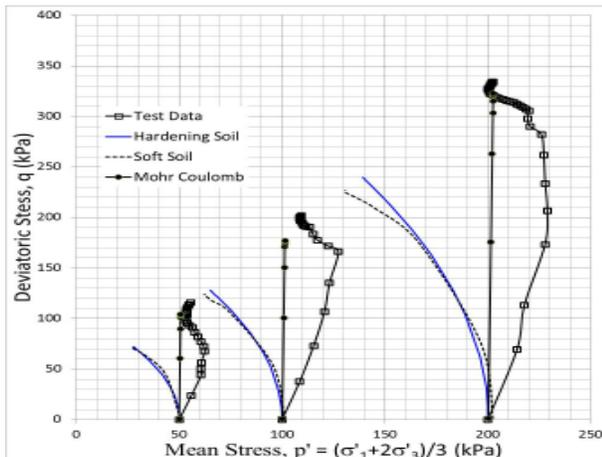
Fig. 16 Stress Paths of Various Soil Models vs. Actual Data
