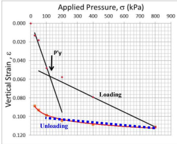
Fig. 11 Oedometer Test for Derivation of  $E_{oed}$
