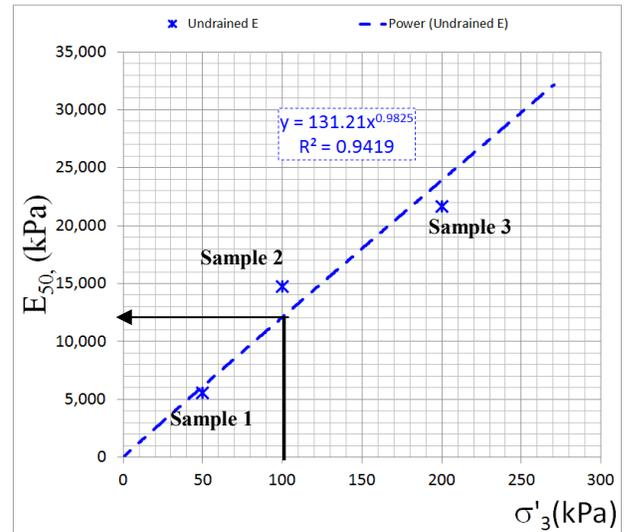
Fig. 7 Determination of  $E_{50}^{ref}$  ( $E_{50}$  at  $P_{ref} = 100$  kPa)
