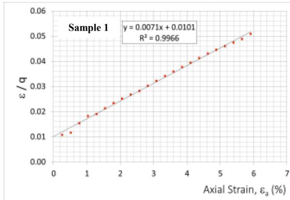
Fig. 9 Derivation of Hyperbolic Parameters of Sample 1
