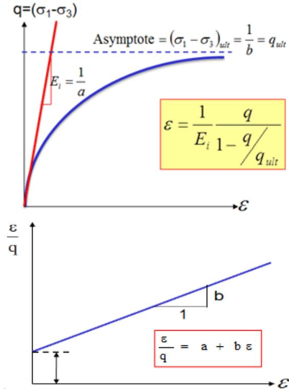
Fig. 8 Process to develop Hyperbolic Equation
