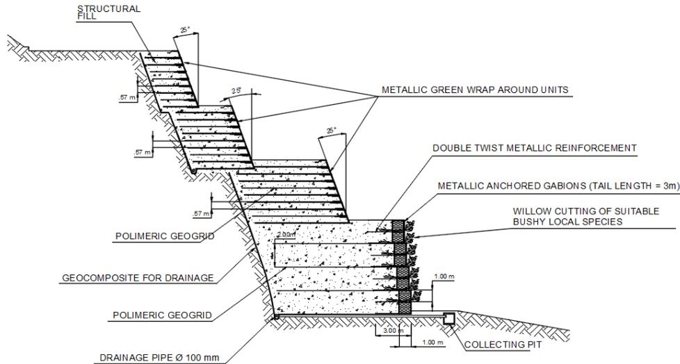
**Figure 2:** Typical section of a reinforced soil slope combining polymeric reinforcements (geogrids) and metallic reinforcements (anchored gabions and steel wrap around units)
