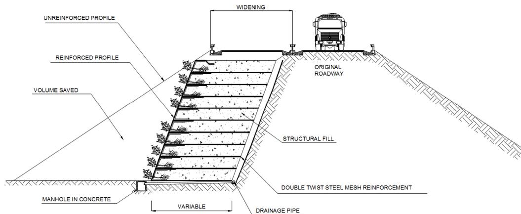
**Figure 1:** Comparison between a reinforced soil slope and an unreinforced one
