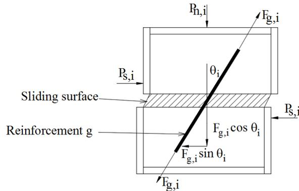
**Figure 8:** Soil element with a reinforcement  $g$  crossing a sliding surface
