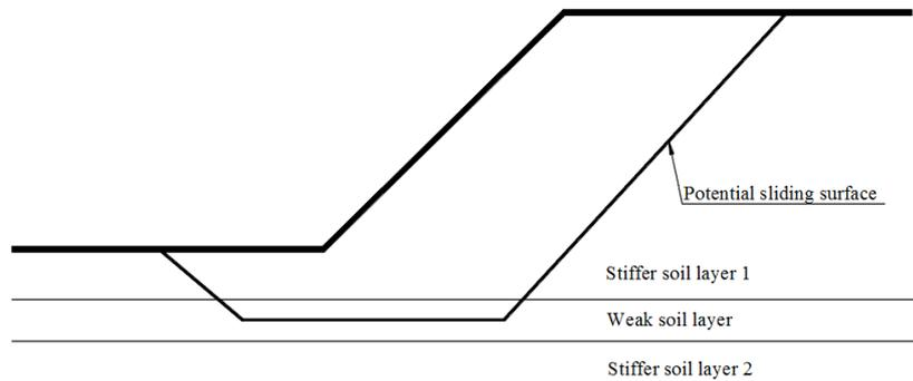
**Figure 6:** Potential polygonal shaped failure mechanism investigated with Janbu method
