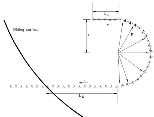
**Figure 10:** Model used to calculate the contribution of the facing of wrapped reinforcing elements
