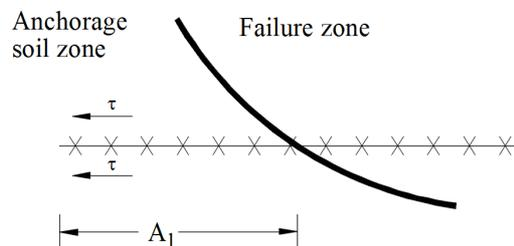
**Figure 9:** Detail of the reinforcement anchorage length  $A_1$
