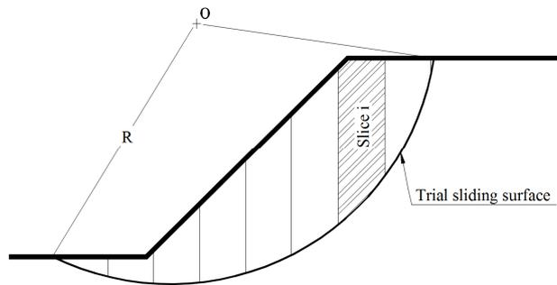
**Figure 4:** Slope cutting in vertical slices, following a circular sliding surface
