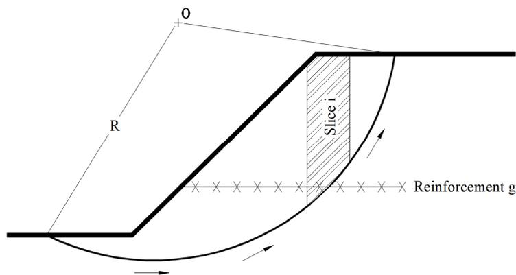
**Figure 7:** Reinforcing element  $g$  intercepting a circular sliding surface
