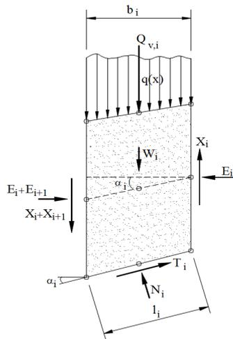
**Figure 5:** Forces acting on a generic slice *i*
