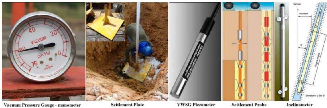
Figure 13. Monitoring instrument used in vacuum preloading
